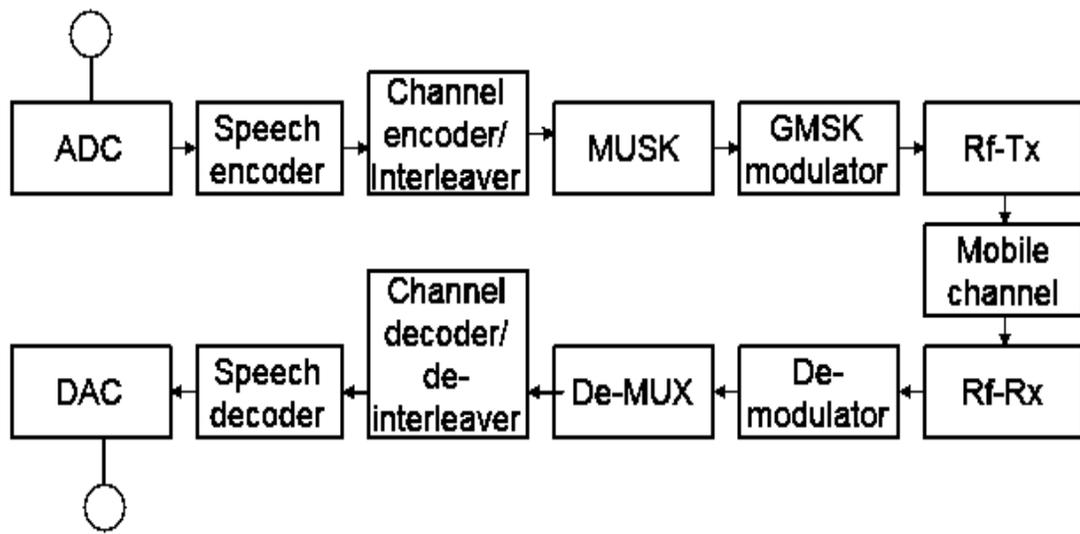
Figure 1: Block diagram illustrating the data structure of the implemented GSM
