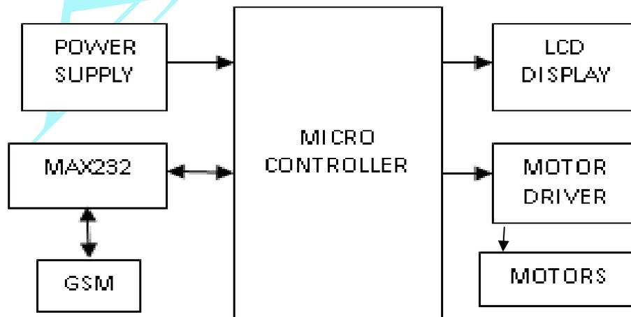
Figure 10: controlling system block diagram.
