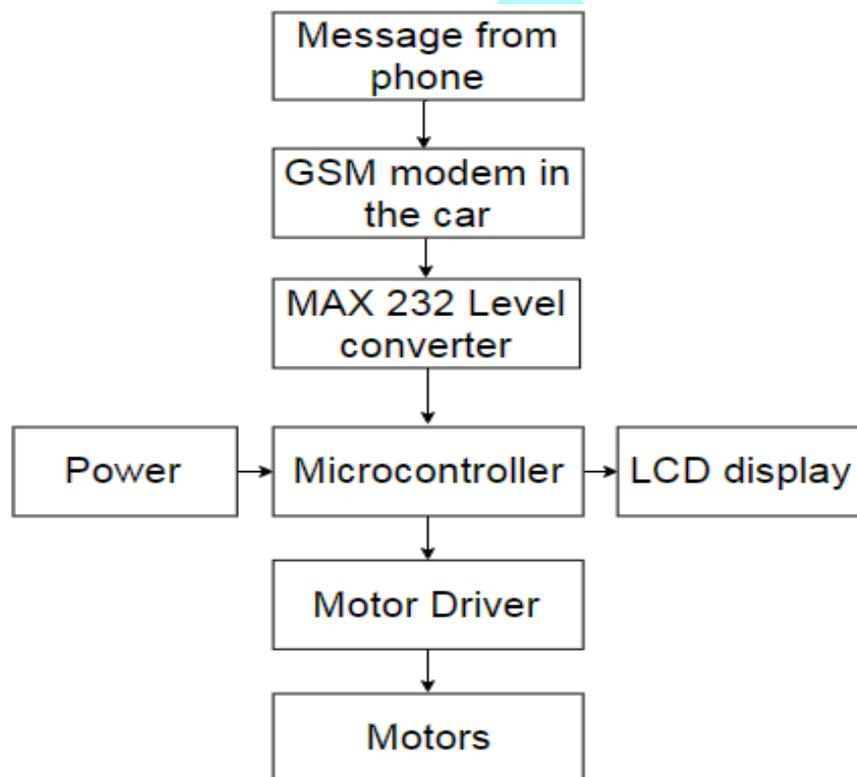
Figure 4: GSM controller based car system flow chart
