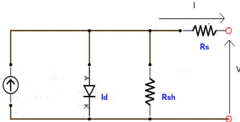
Figure 2: Solar cell and PV device equivalent circuit
