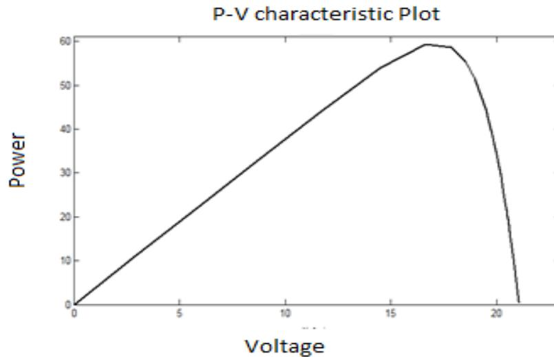
Figure 7: PV characteristic graph
