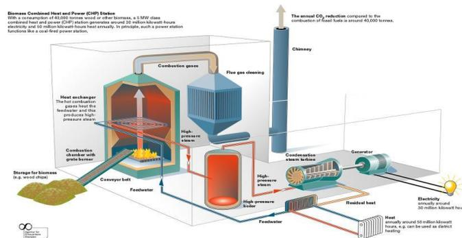
**Figure 1: Biomass power generation using a steam turbine**
