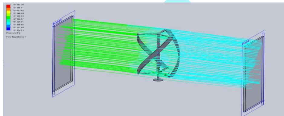
Figure 5 Isometric view of flow simulation (VAWT)
