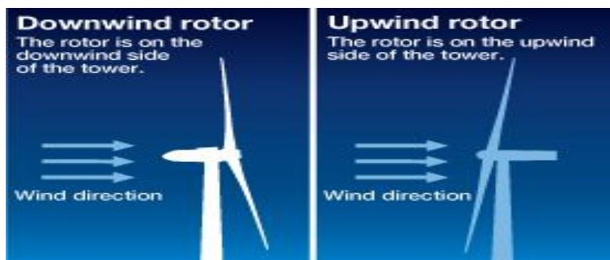
**Figure 2 Upwind and Downwind Rotor**
