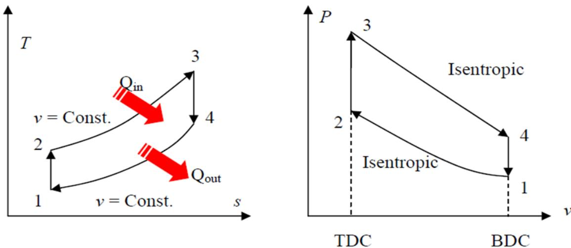
Figure 4: T-s & P-v diagram of Ideal Otto cycle
