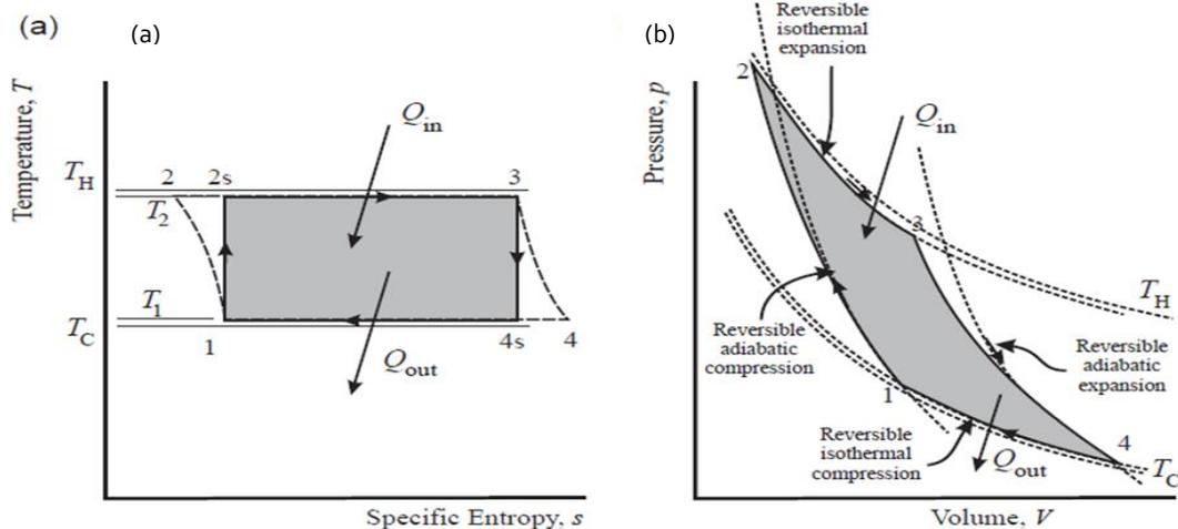
Figure 1: (a) T-s and (b) P-v diagram of Carnot cycle
