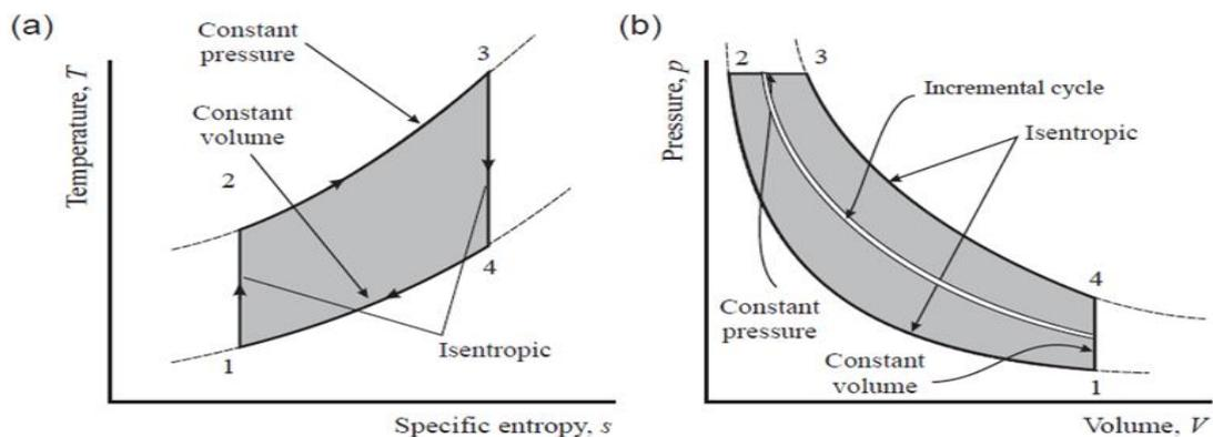
Figure 6: T-s & P-v diagram of Ideal Diesel cycle
