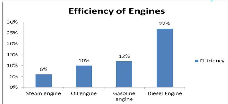
Figure 7: Average Efficiencies of Engines
