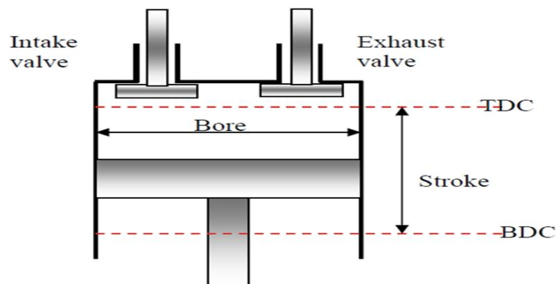
Figure 3: Piston & Cylinder
