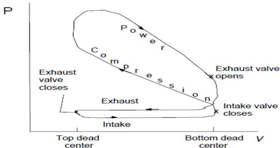
Figure 5: Actual Otto engine Cycle (Includes air intake and air removal)
