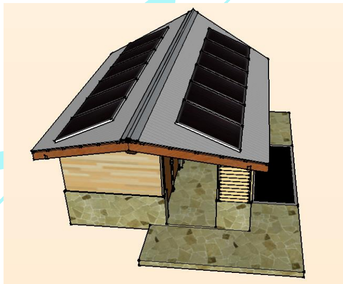
Figure 6: Installation of Solar Panel on the Shower Room
